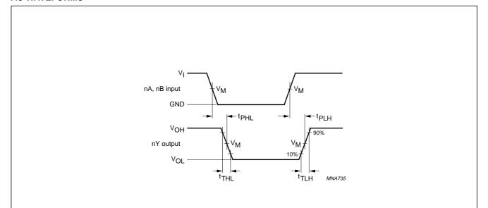
For 74HC2G32:  $V_M$  = 50%;  $V_I$  = GND to  $V_{CC}$ . For 74HCT2G32:  $V_M$  = 1.3 V;  $V_I$  = GND to 3.0 V.
